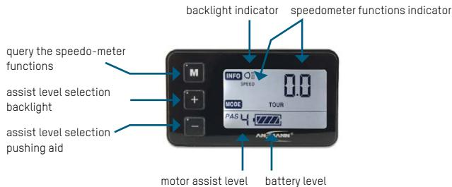
When the electric drive was switched ON at the battery the motor assist level 2 is automatically preselected. With the buttons “-” und “+” the motor assist levels could be changed to level 0 (no motor assist) and from level 1 to level 6.
