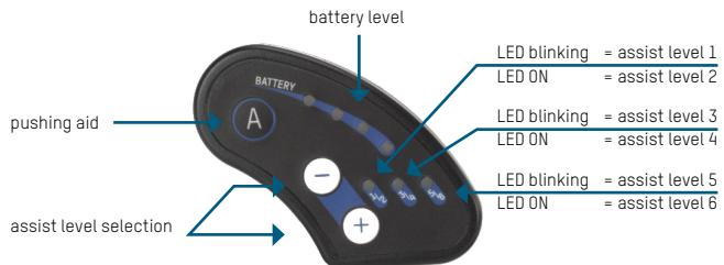
When the electric drive was switched on at the battery the motor assist level 2 is automatically preselected. With the buttons " - " und " + " the motor assist levels could be changed to level 0 (no motor assist) and from level 1 to level 6. Depends on the selected motor assist level you will get different motor speed (cruise control function). When you press the button " A " the motor will give a speed of max. 6km/h without pedaling (pushing aid function) as long as you press this button.
