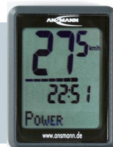
The higher the level of the electric motor support, the lower the range with one battery charge. By pushing the lower button (U) several times the level of the Pedelec support can be turned down from the POWER level to the OFF MODE.
