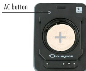
After installing the battery there are some settings to choose. When the battery is assembled the words "AKKU AN?" appear in the bottom line of the display. When "ANSMANN" (Sleep Mode) or nothing appears, turn the device on by pushing the "AC" button on the back of the device. Put the Bicycle computer into its holder and attach holder to the bicycle. Make sure that it is locked in place. To get to the settings push the button (M) in the middle on the operating unit and hold it for 3 Seconds.
