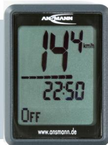
Turn on the Pedelec support by pushing the upper button (0) and switch up through the support levels ECO/ ECO+/ NORMAL/ NORMAL+/POWER pushing the (0) button again.
