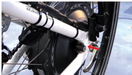
Correct position of the torque support on the pedelec
