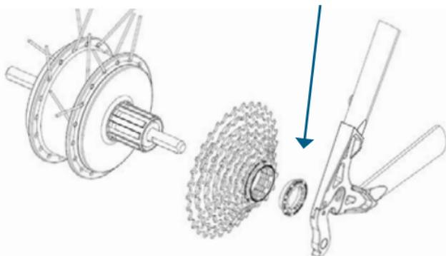
When fastening the impeller, make sure the moulded part of the torque supports (both side) is turned downwards, that the axis fits correctly inside the fork (front wheel motor) / back end (rear wheel motor). The tightening torque of the axle nuts is 25Nm.
