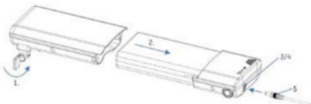
To charge the battery, open the cap (3) on the charging socket (4) and connect the plug (5) from the charger.
